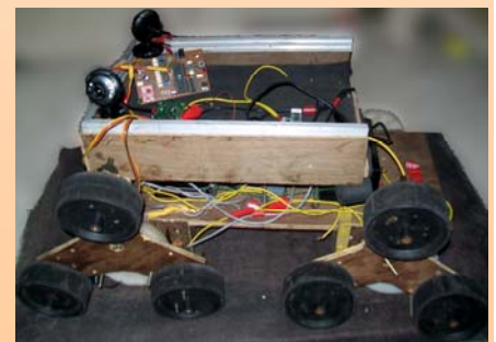
Fig. 1 Mobile Autonomous Robot
