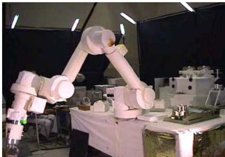
Figure 3: ETS-7 Robotic Arm during ground testing 8
