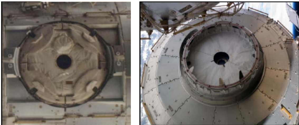
Fig 8: Active and passive rings of the common berthing mechanism [17]
